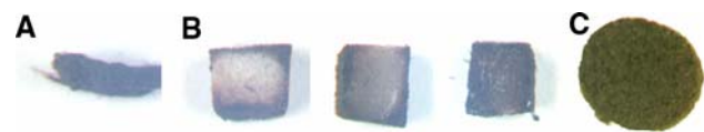
Fig. 6 Ink absorption in (a) silk non-woven structure, (b) three different partially dissolved silk scaffolds and in (c) salt-leached scaffold
